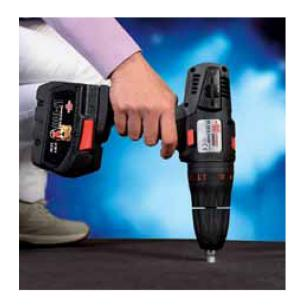
Control of vertical movement by means of a standard electric or battery screwer, introduced into a small central hole in the floor.
